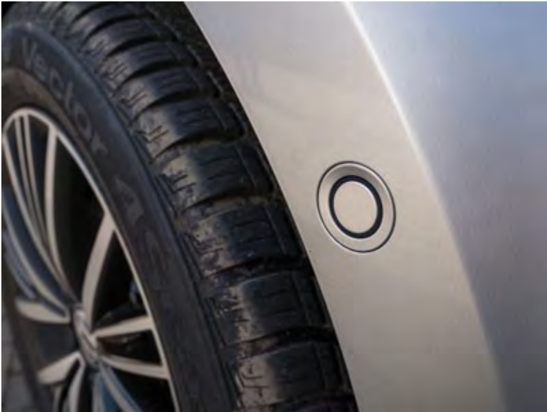
Figure 4. An ultrasonic sensor on the edge of a wheel well opening. (Image: Wikipedia, Basotxerri, CC BY-SA 4.0)
