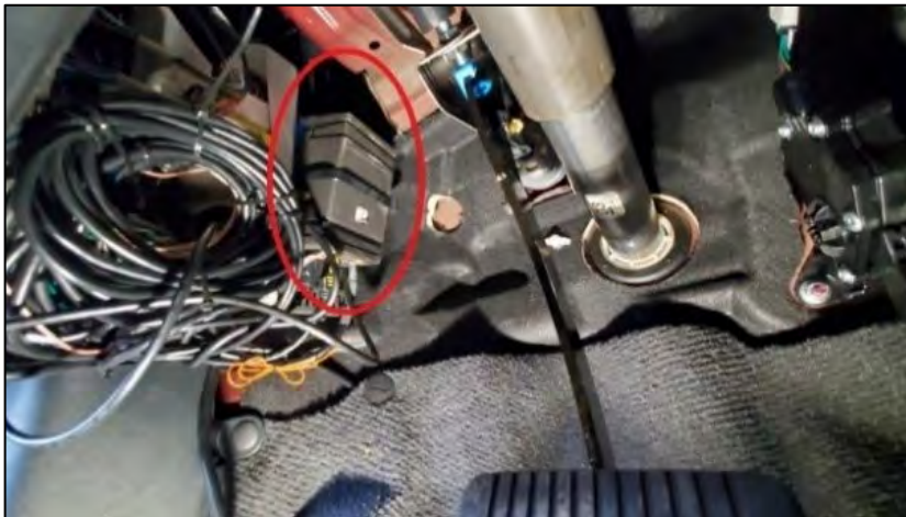
Figure 13. Main unit of the VTTI DAS mounted in the driver's footwell.
