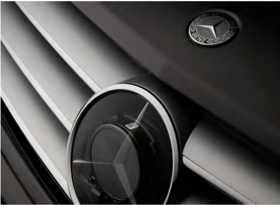
Figure 3. This “see through” image shows how a radar sensor may be positioned behind a solid plastic cover in the grille. (Image: Mercedes-Benz)
